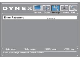
**4** Press the number buttons to enter the four-digit password. The *Parental Controls* menu opens.
